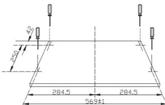
11. Take down the fan-shaped door frames, then fix the left and right fanshaped door frames with the connected plate by 4pcs ST3.5\*8mm countersunk self-tapping screws. See pic below. Fix the fan-shaped door frames on the door with screws. Make sure the frames are symmetrical. Install the door into the cooker hood, the two sides of the door can be pulled to the end and the door can be safely locked. If the door cannot be safely locked, you can release the plastic handle.
