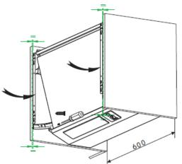
7. Install the outlet as followings: Align the 3 pcs side slots of the outlet with the 3 edges of the blower, insert the 3 edges into the outlet slot, See pic 1,then finish as pic 2 shown.
