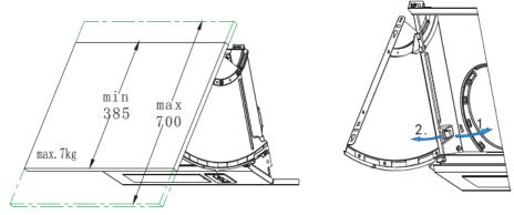
10. Mark the installation position of the door and the size of the fixed screws. If the upper edge of the door is not as high as the upper edge of the cupboards, please adjust the size accordingly. Mark the positions of the screws on the door, and make sure the size is as accurate as  $569 \pm 1$ .
