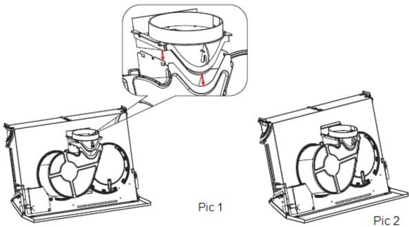
8. Connect the air-outlet board and the air-outlet tube (Vent Hose) which will need to feed through to the outside of the building. Rigid kits, if preferred, can be obtained from either the retailer who supplied the hood, or DIY Stores and Builders Merchants.
