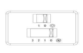
To operate: pull up the front panel, turn on the cooker hood, and then choose the fan speed setting.
