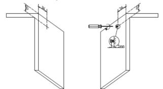
4. Hang the cooker hood on the screws between the two cupboards.
