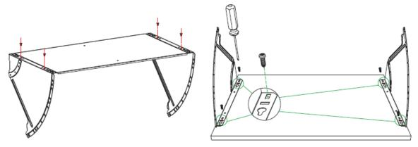
12. The two screws on both sides of the cooker hood can adjust the sliding of the door, according to the weight of the door.
