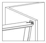
5. Push the fan-shaped door frames to the end, in order to make the outer edges of the door frames at the same vertical level as the outer edge of the cupboards.
