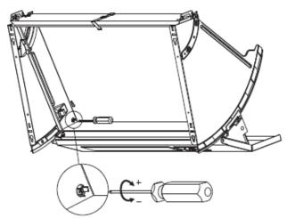
13. Install the adjusting plate, in order to cover the gap between the wall and the bottom of the cooker hood.
