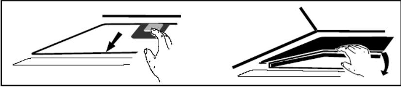
Plug the activated carbon filter into the unit and turn it in clockwise direction. Repeat the same on the other side.
