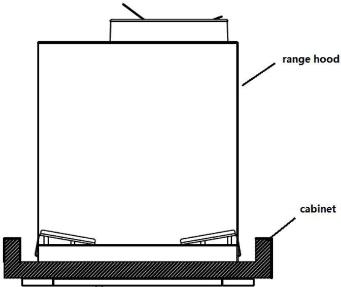
2. Remove 8 screws of 4 hanging plates on the range hood, push the 4 hanging plates on the top side of cabinet edge.
